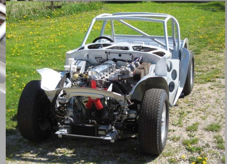
The bodywork is recieving final adjustments and preparations before painting. We hope to have the car fully assembled and ready for track-tests within a month.
