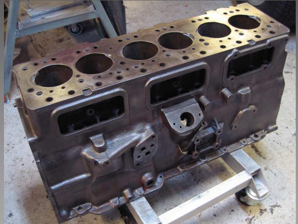
*The new engine block ready for machining.*
