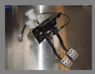
All suspension, brakes, steering etc has been disassembled and inspected for wear and possible damage. Most bits are now lying on the shelves ready for assembly. Some parts has also received modification in order to improve stability and precision such as the pedal-assembly and the tie bar keeping the engine and gearbox in place.
