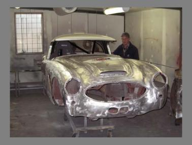
Work on the new chassis will start very soon. All panels, bonnet, boot and shrouds have been stripped to bare metal and ready for Austin-Healey specialist Bengt Larsson's experienced craftsmanship. Probably the best man there is in Sweden for this job! A new welded in roll-cage will be fitted for strength and safety. The complete chassis and bodywork will then be painted, ready for assembly with all other bits in April.
